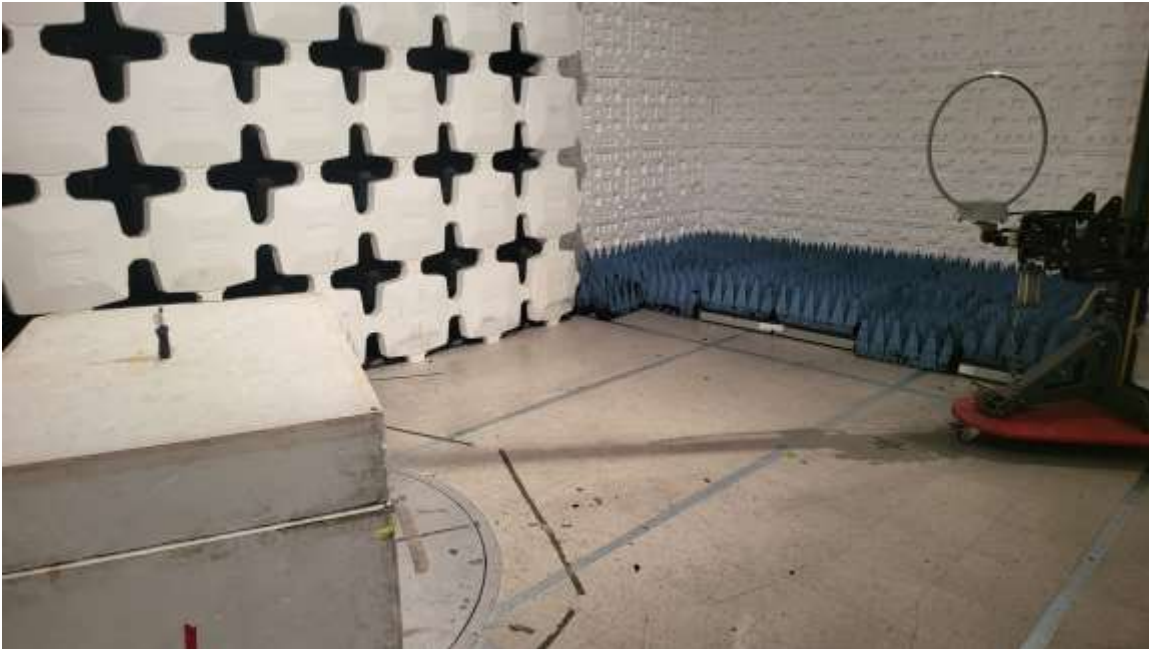
Figure 2. Radiated Emissions Test Setup, .15 MHz to 300 MHz, 1.0-mile (300-3445)
