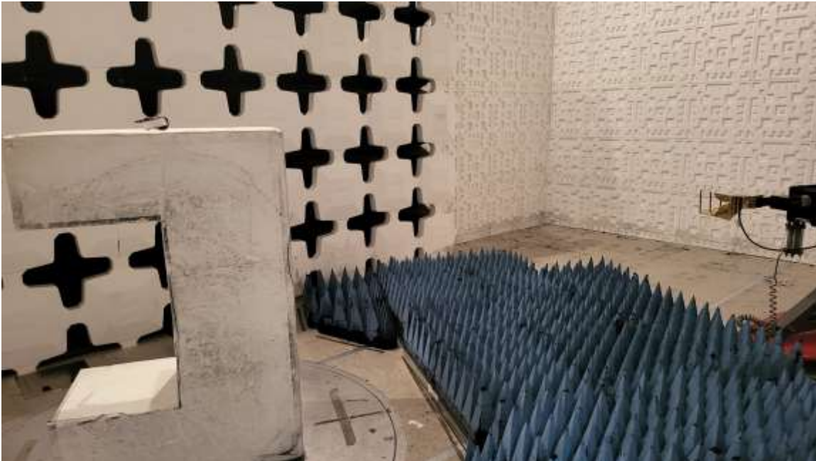
Figure 5. Radiated Emission Test Setup, above 1 GHz, 1.0-mile (300-3445)
