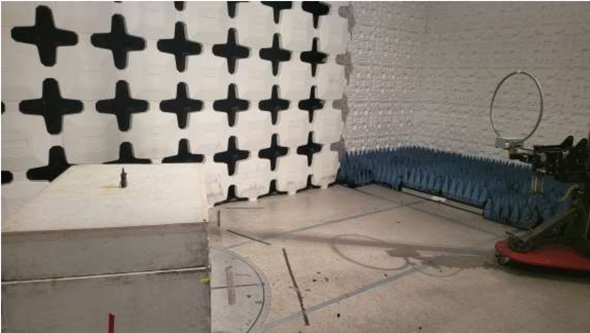
Figure 2. Radiated Emissions Test Setup, .15 MHz to 300 MHz, 0.5-mile (300-34451-1)
