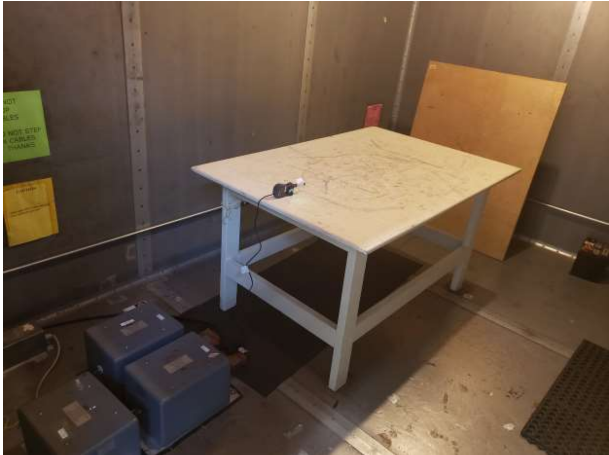
Figure 6. Conducted Emissions Test Setup
