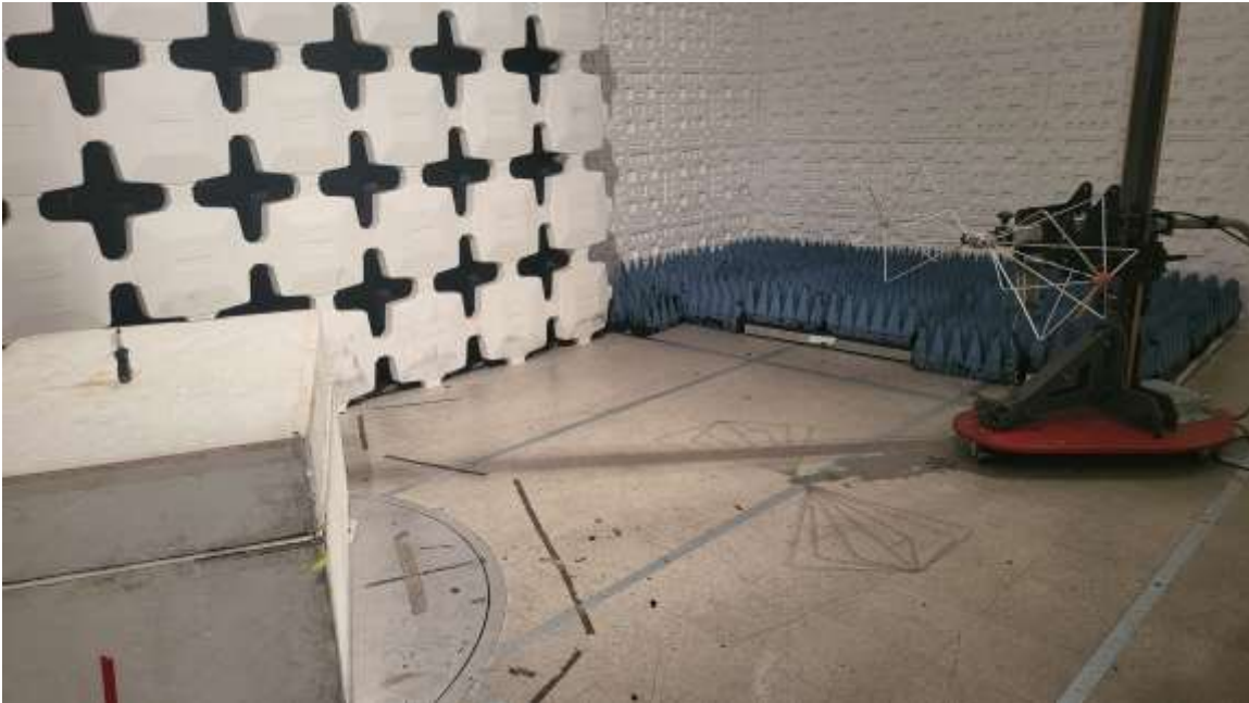
Figure 3. Radiated Emissions Test Setup, 30 MHz to 200 MHz, 1.0-mile (300-3445)
