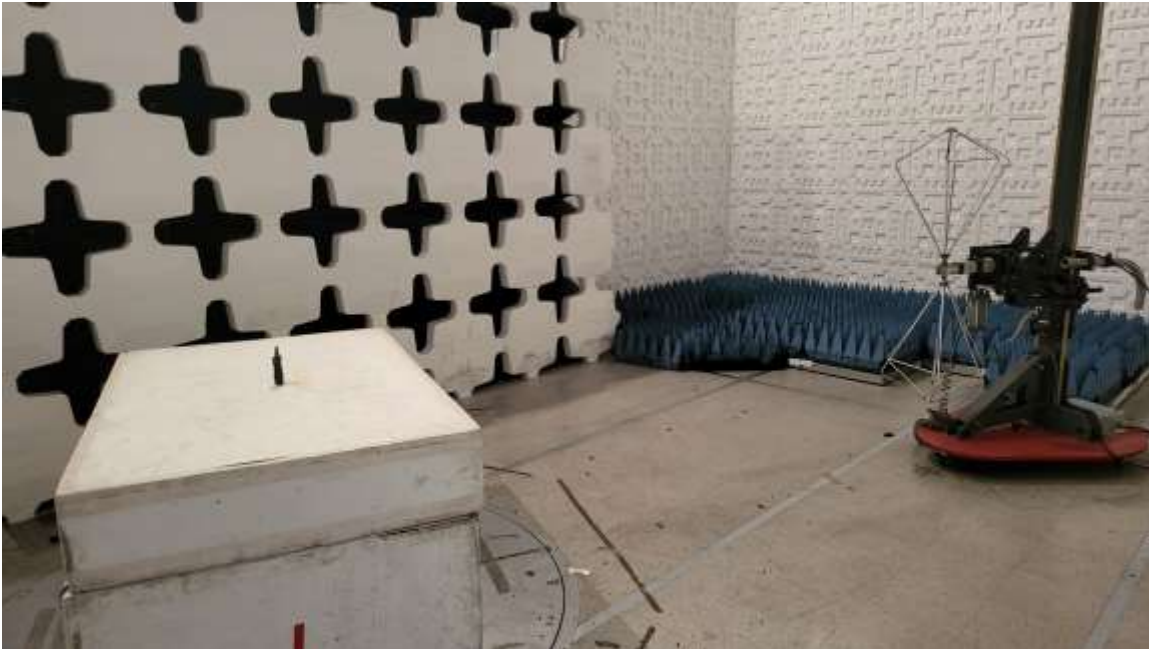
Figure 3. Radiated Emissions Test Setup, 30 MHz to 200 MHz, 0.5-mile (300-34451-1)
