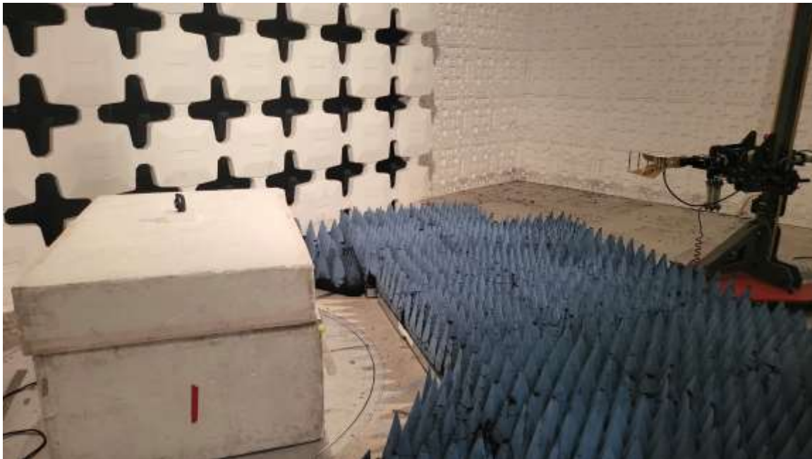
Figure 5. Radiated Emission Test Setup, above 1 GHz, Back
