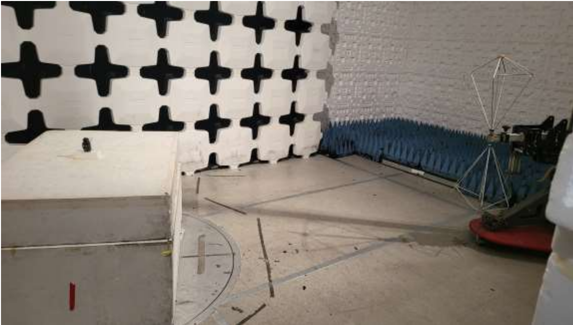
Figure 3. Radiated Emissions Test Setup, 30 MHz to 200 MHz, Back
