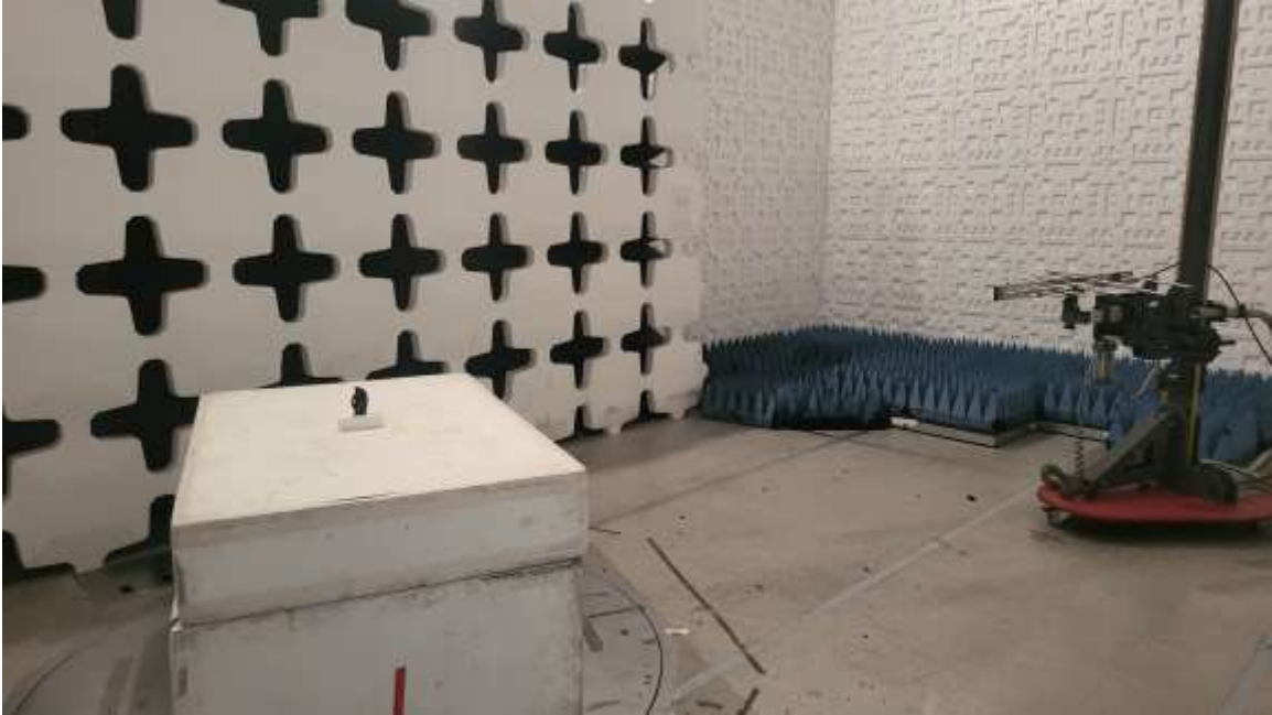
Figure 4. Radiated Emissions Test Setup, 200 MHz to 1GHz, Back
