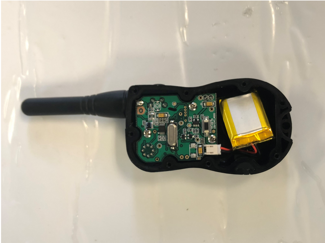
Figure 1. EUT cover removed
