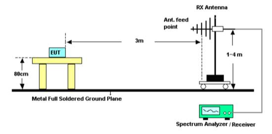
(C) Radiated Emission Test-Up Frequency Above 1GHz
