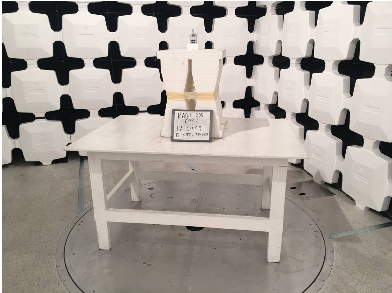
Figure 5. Radiated Emissions Test Setup, above 1 GHz, Close-up
