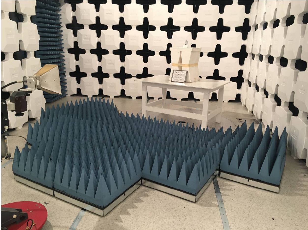
Figure 6. Radiated Emissions Test Setup, above 1 GHz with Antenna
