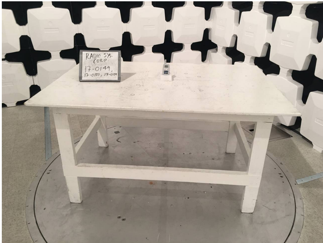
Figure 1. Radiated Emissions Test Setup
