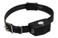
The GPS 3.0 Mobile Collar Unit requests GPS assistance data from and provides status information to reference Base Units. To extend its battery life, the Collar Unit's radio is active only when necessary. Under certain conditions it will also stop navigation in order to conserve power and extend battery life. Motion is required to re-start navigation.
