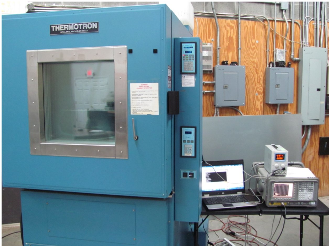
Figure 7. Frequency Stability Testing
