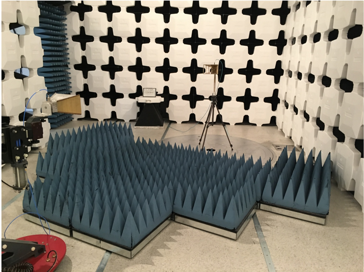
Figure 6. Substitution Setup (above 1 GHz)
