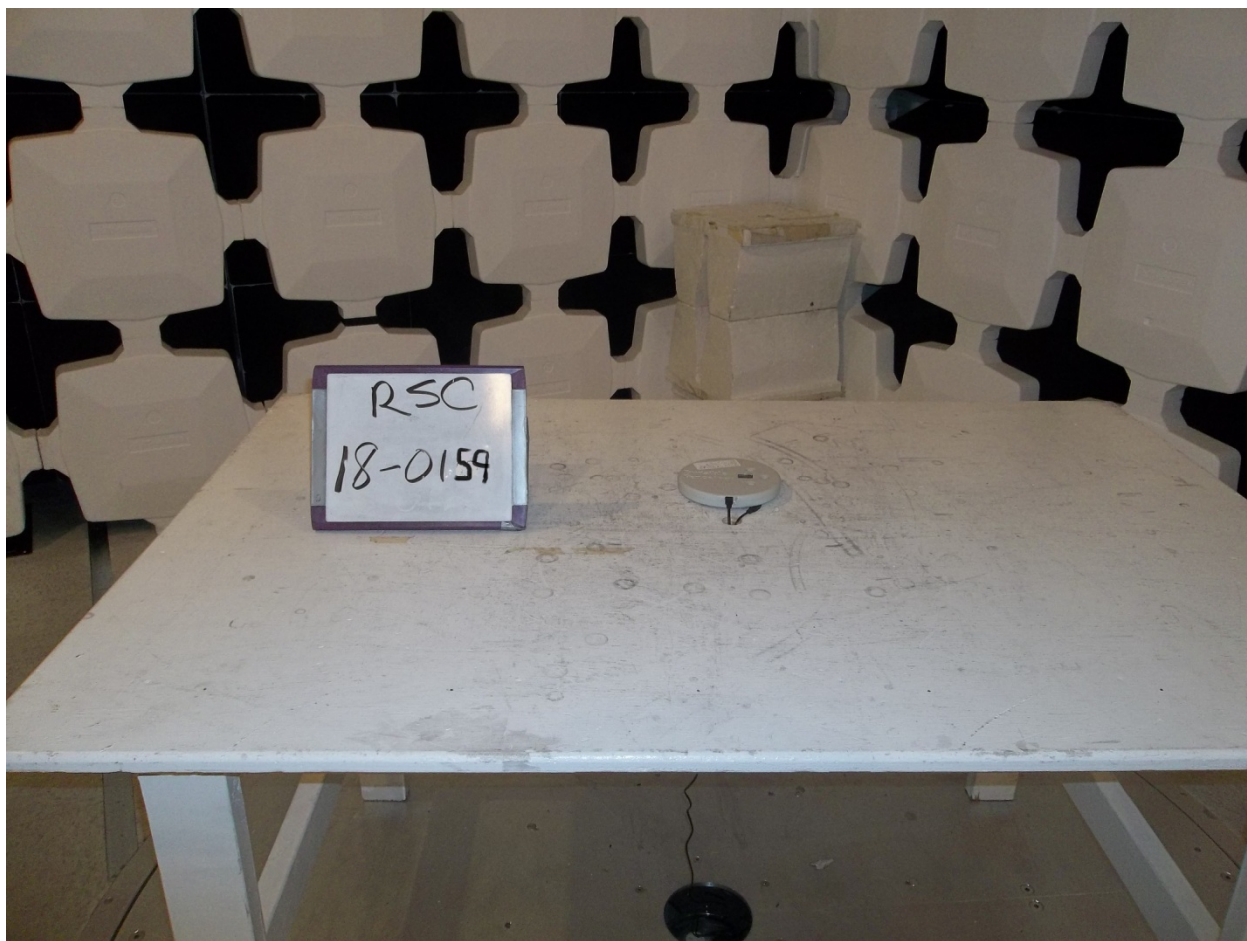
Figure 1. EUT Radiated Emissions Test Setup
