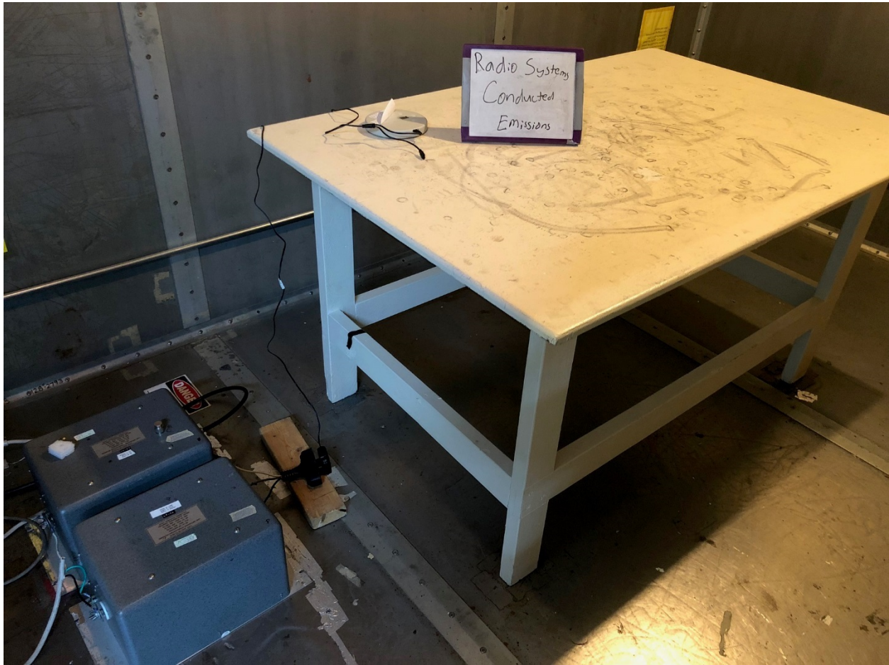
Figure 7. Powerline Conducted Emissions Test Configuration
