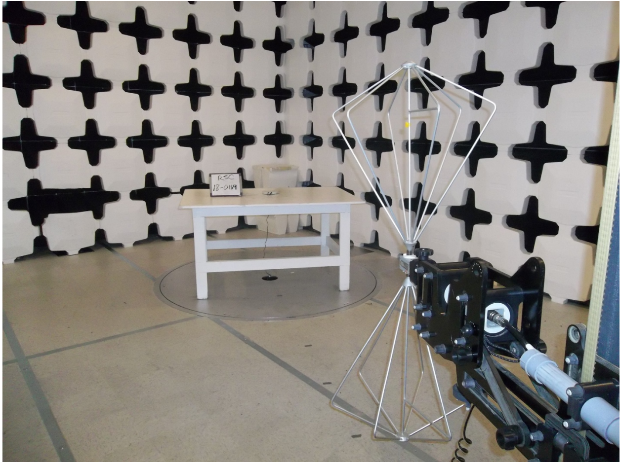
Figure 5. Radiated Emissions, 30-200 MHz
