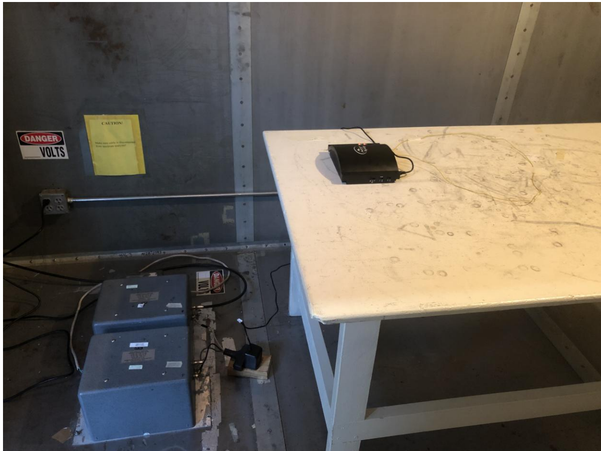
Figure 5. Power Line Conducted Emissions Test Setup
