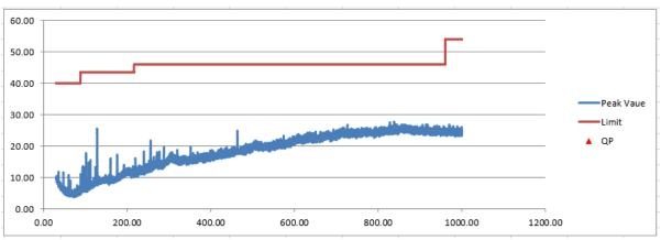
Figure 3. Radiated Emissions Graphical Data, 30-1000 MHz – Horizontal
