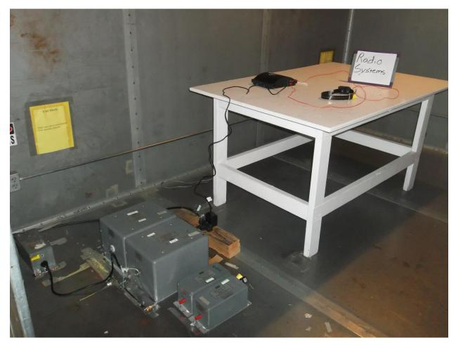
Figure 5. Power Line Conducted Emissions Test Setup
