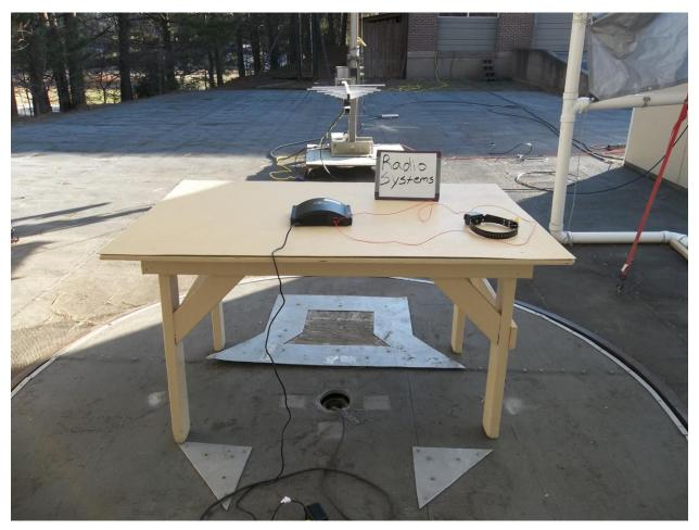
Figure 4. Radiated Emissions Test Setup (200 Mhz - 1 GHz)
