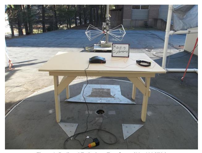
Figure 3. Radiated Emissions Test Setup (30 - 200 MHz)
