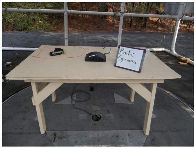
Figure 1. Radiated Emissions Test Setup
