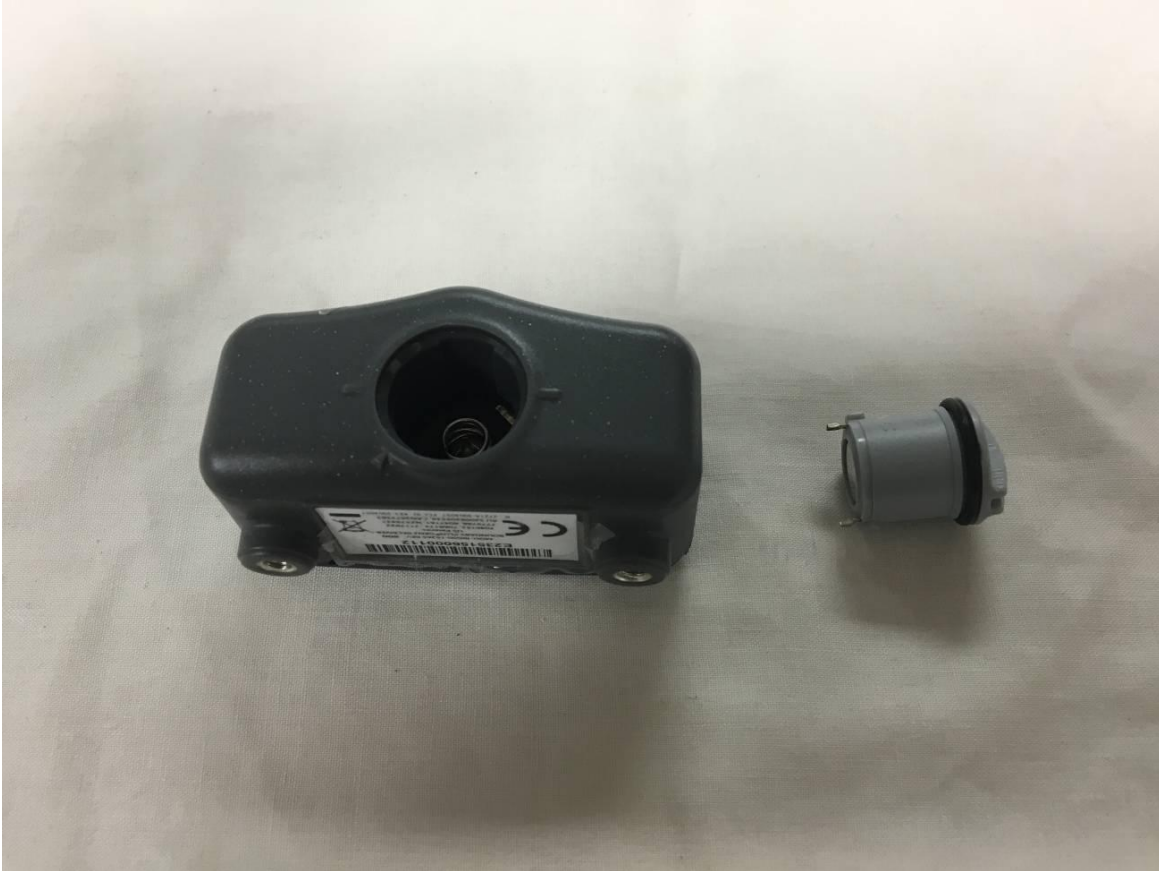
Figure 6. Battery Pack Removed
