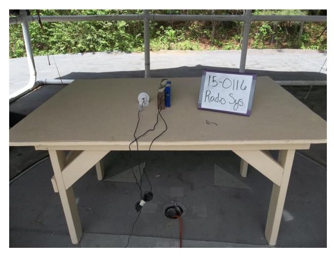
Figure 1. Radiated Emissions Test Setup, Front (Radio Test with EUT in worst case position)
