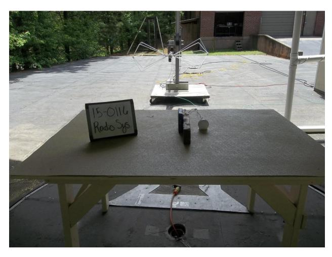
Figure 3. Radiated Emissions Test Setup, Rear 30 MHz to 200 MHz (Radio Test with EUT in worst case position)
