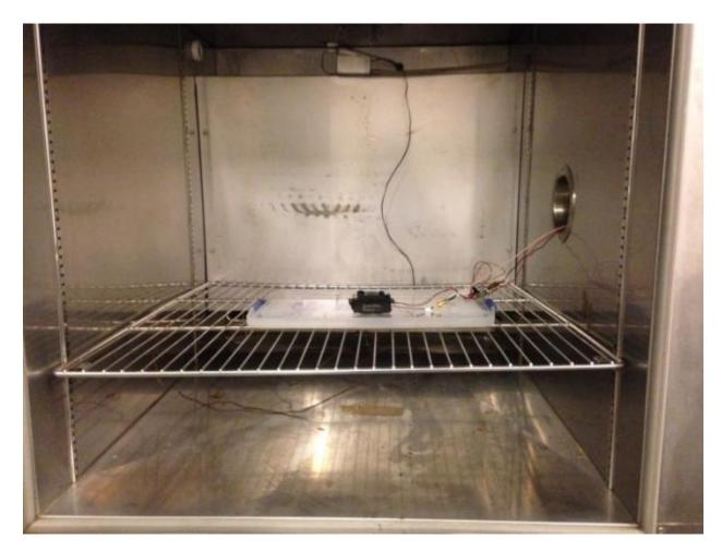
Figure 6. Frequency Stability Test Setup
