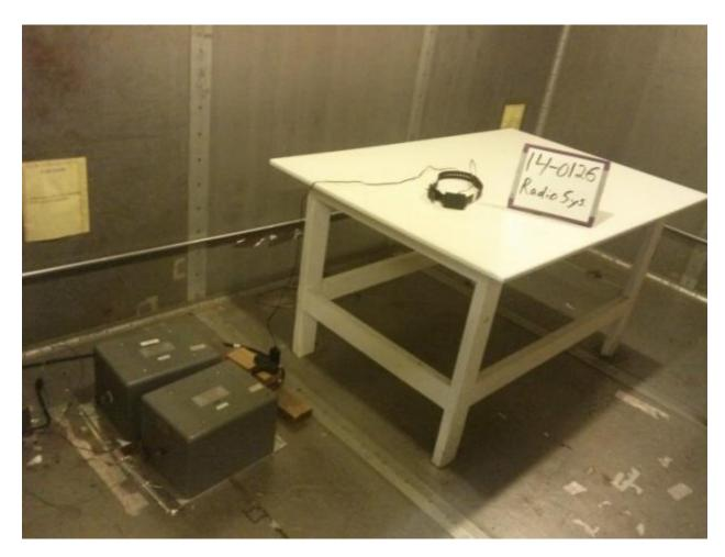
**Figure 5. Powerline Conducted Emissions**
