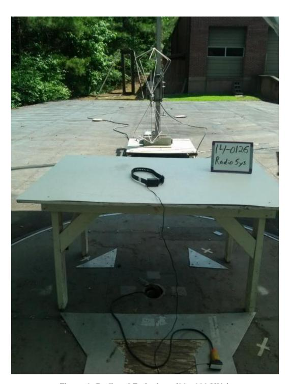
Figure 3. Radiated Emissions (30 - 200 MHz)
