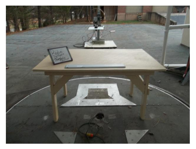
Figure 2. Radiated Emissions Test Setup, .09 MHz to 300 MHz, Back
