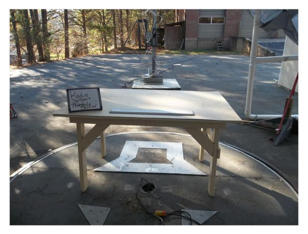
Figure 3. Radiated Emissions Test Setup, 30 MHz to 200 MHz, Back
