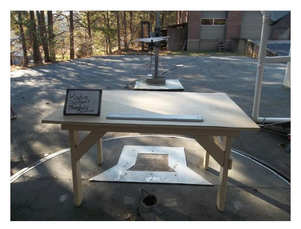
Figure 4. Radiated Emissions Test Setup, 200 MHz to 1GHz, Back
