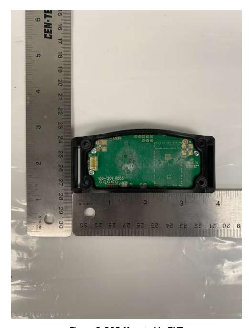
Figure 5. PCB Mounted in EUT
