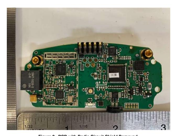
Figure 9. PCB with Radio Circuit Shield Removed
