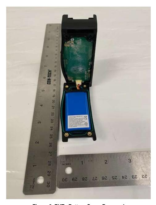
Figure 2. EUT- Battery Cover Removed
