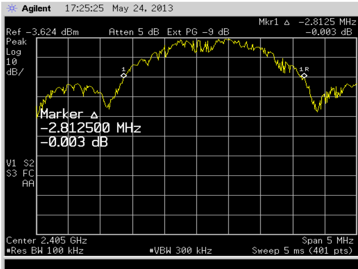
Figure 36. Low Channel 99% Bandwidth
