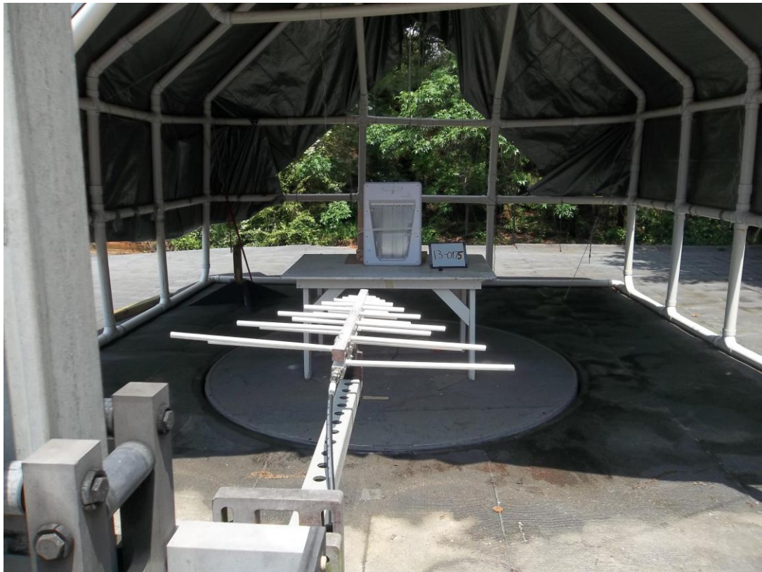
Figure 5. Front View with Log-Periodic Antenna
