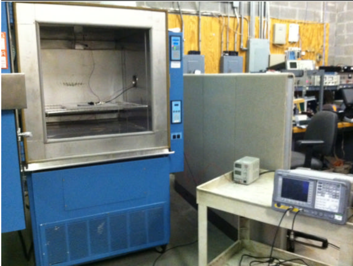
Figure 4- Frequency Stability Test Setup
