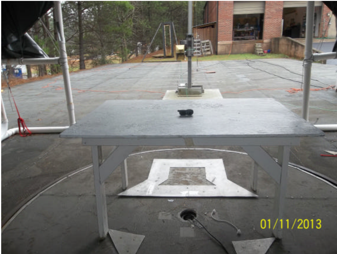
Figure 3- Radiated Emissions Test Setup (below 1000 MHz)
