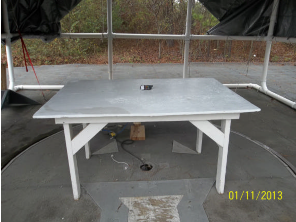
Figure 1- Radiated Emissions Test Setup
