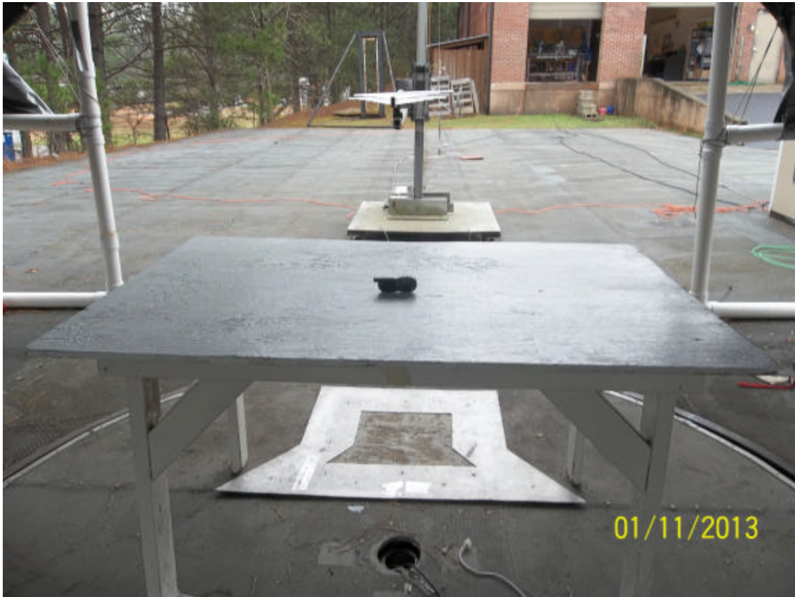
Figure 2- Radiated Emissions Test Setup (below 1000 MHz)
