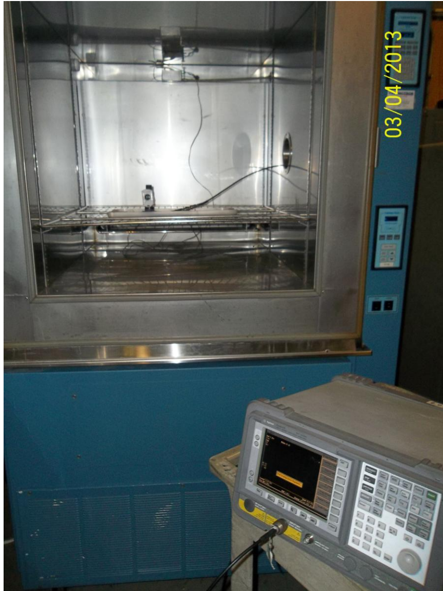
Figure 6- Frequency Stability Test Setup
