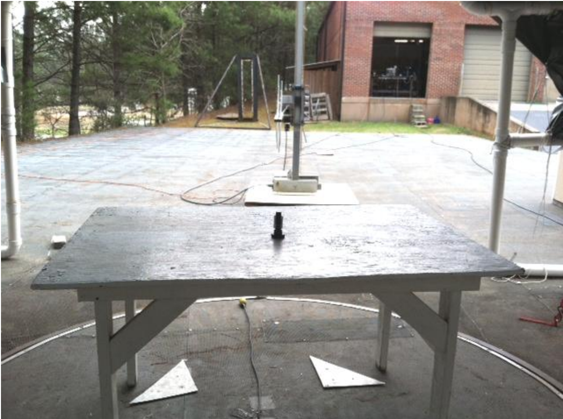
Figure 4. Radiated Emissions Test Setup (between 200 - 1000 MHz)
