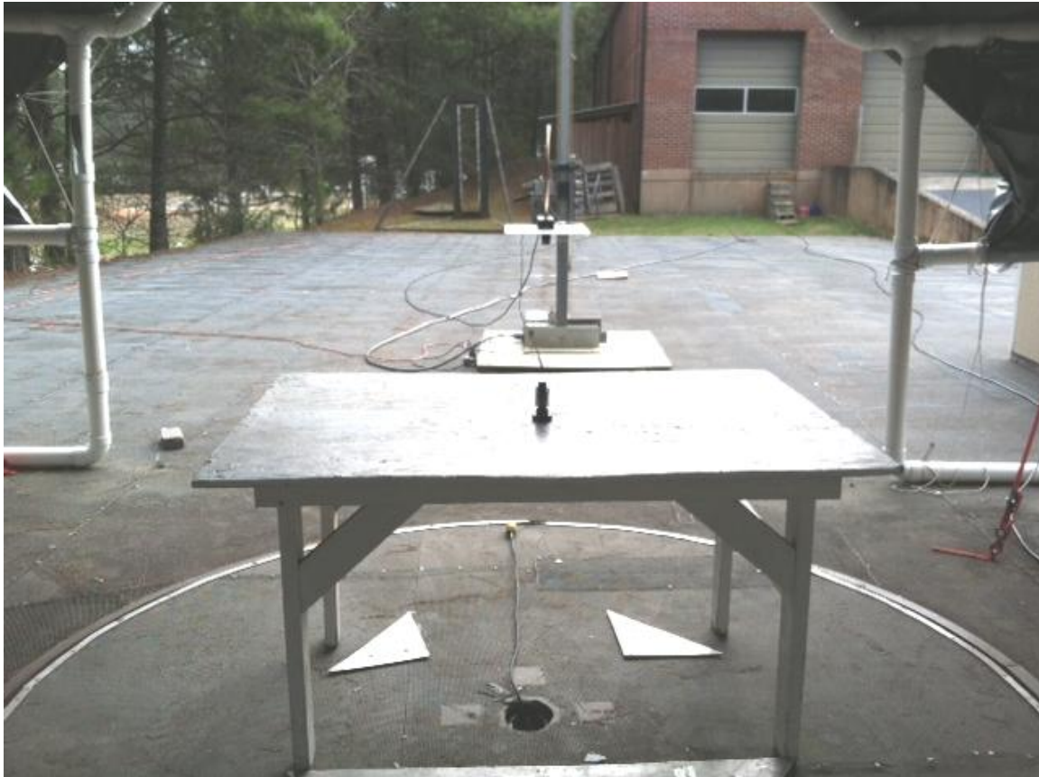
Figure 2- Radiated Emissions Test Setup (below 30 MHz)
