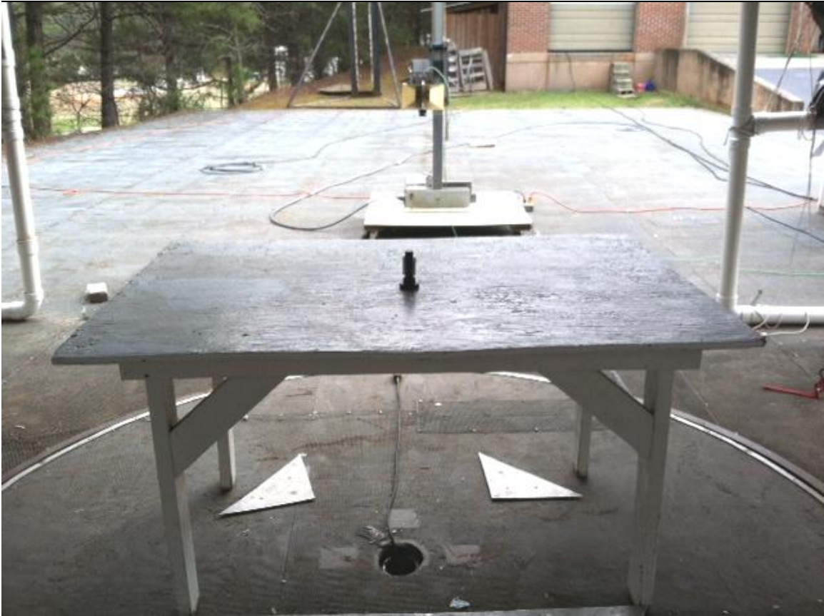
Figure 5. Radiated Emissions Test Setup (between 1000 - 5000 MHz)
