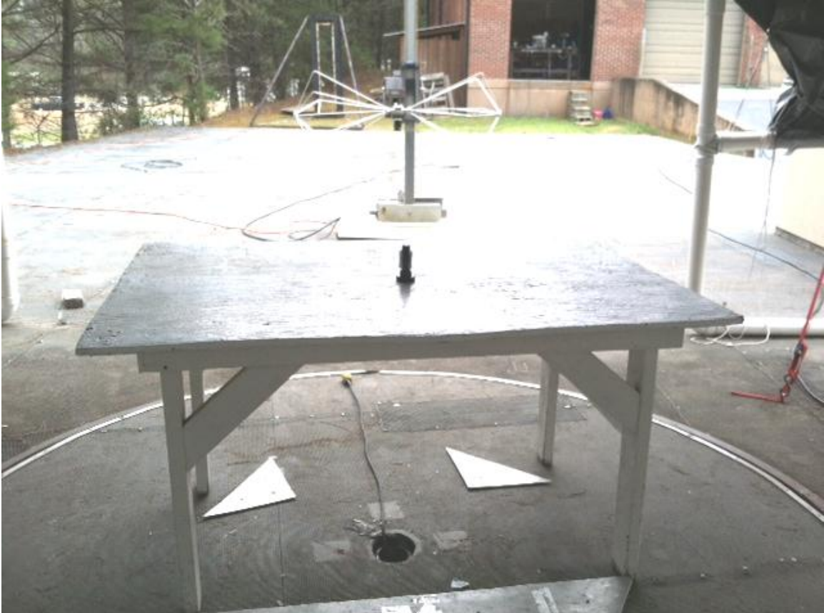
Figure 3- Radiated Emissions Test Setup (between 30 - 200 MHz)
