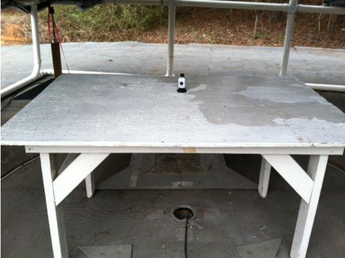
Figure 1- Radiated Emissions Test Setup
