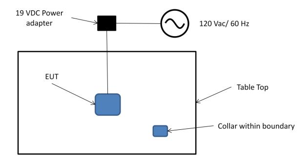
Figure 2. Block Diagram of Test Configuration
