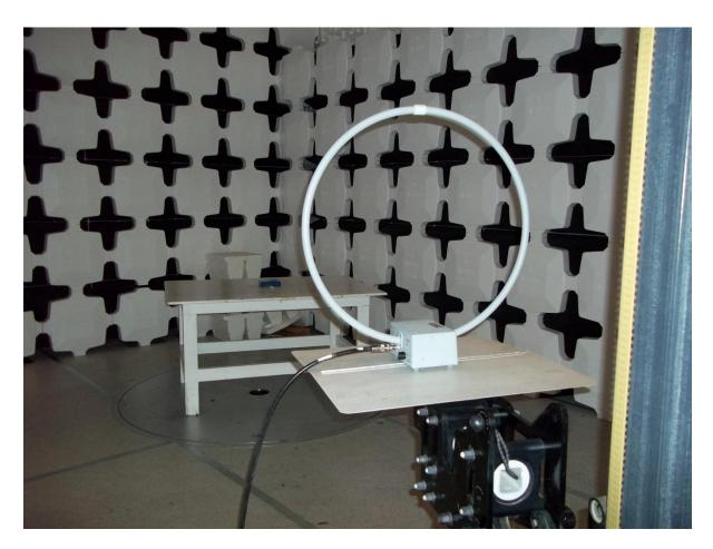
Figure 6. Radiated Emissions Test Setup, 9 kHz - 30 MHz
