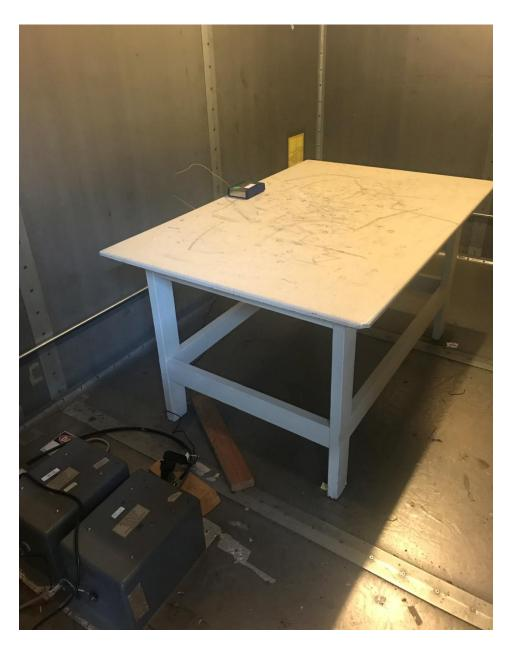
Figure 5. AC Powerline Conducted Emissions Test Setup
