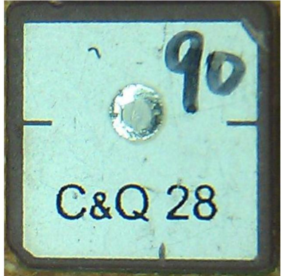
Bondale GPS antenna (Mobile Unit)
