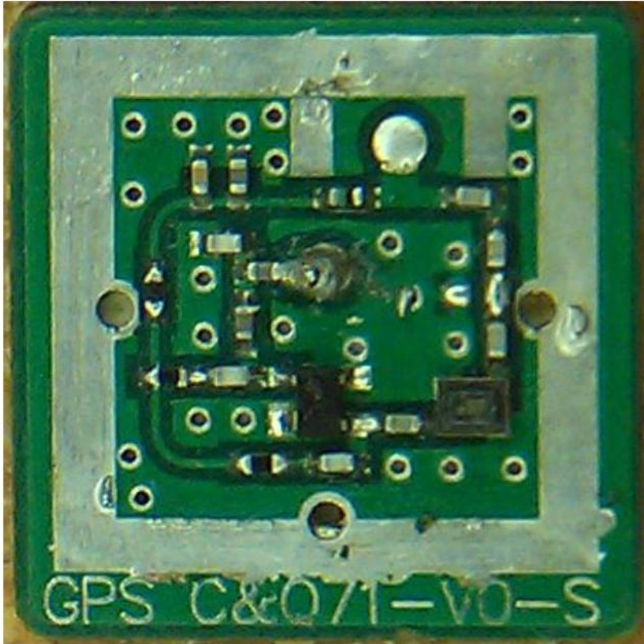
Bondale GPS antenna (Mobile Unit)
