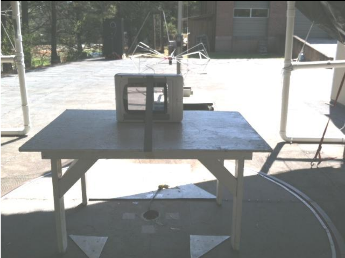
Figure 3- Radiated Emissions, Low Frequency (BiCon)
