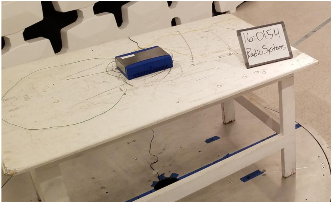
Figure 1. Radiated Emissions Test Setup
