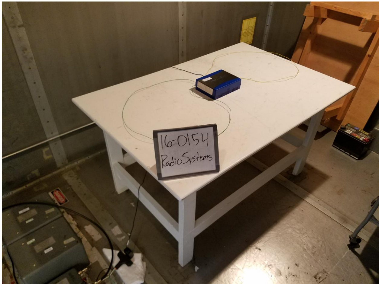
Figure 5. Power Line Conducted Emissions Test Setup
