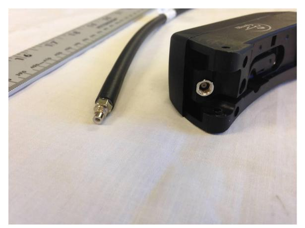
Figure 8. EUT, Unique Antenna Connector
