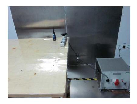
2.2 Photograph – Radiation Emission Test Setup Below 30MHz
