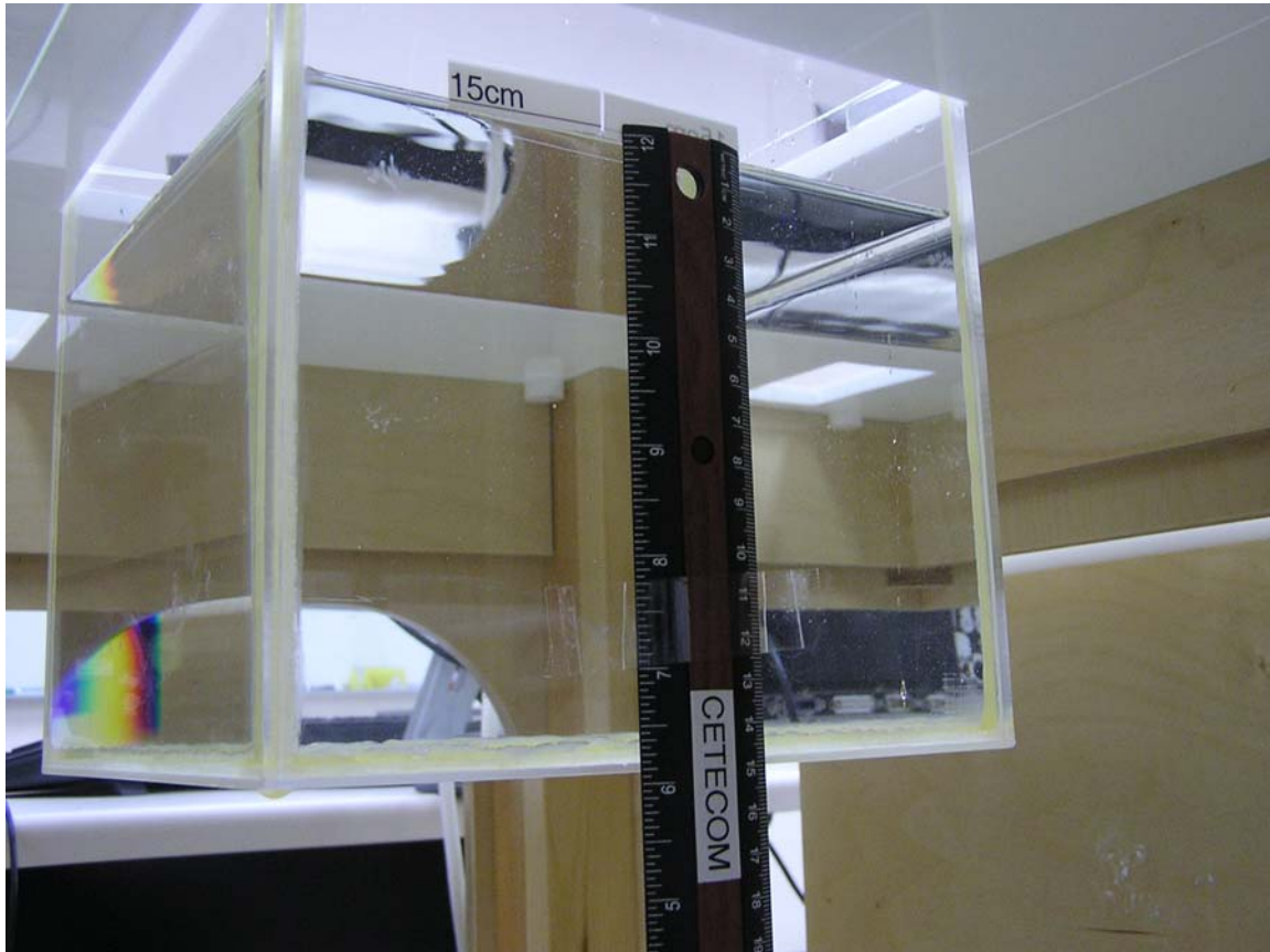
Photo 2. Photo to demonstrate 15 cm Z-axis flat phantom
