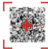
Figure 20 Imager Bracketed Crosshair Target on 2D Barcode
