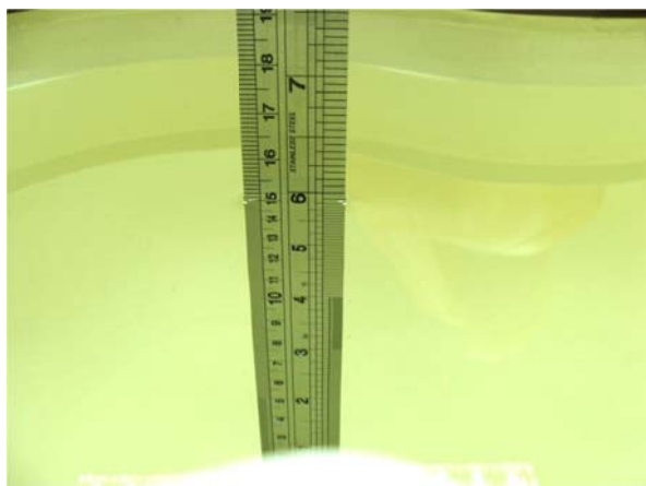
Fig 6.1 Photo of Liquid Height for Head SAR
