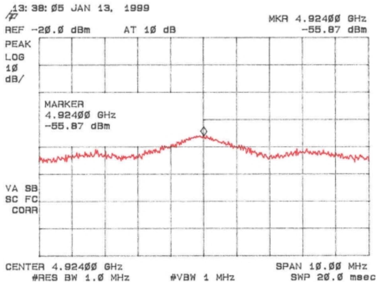
**TABLE 4d PEAK RADIATED SPURIOUS EMISSIONS (Low) – Omni Antenna**
