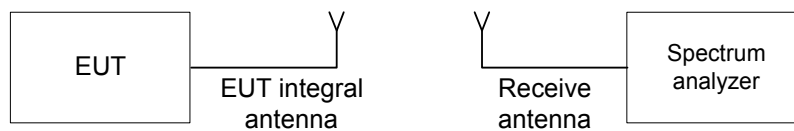
Figure 7.1.1 Setup for transmitter shut down test
