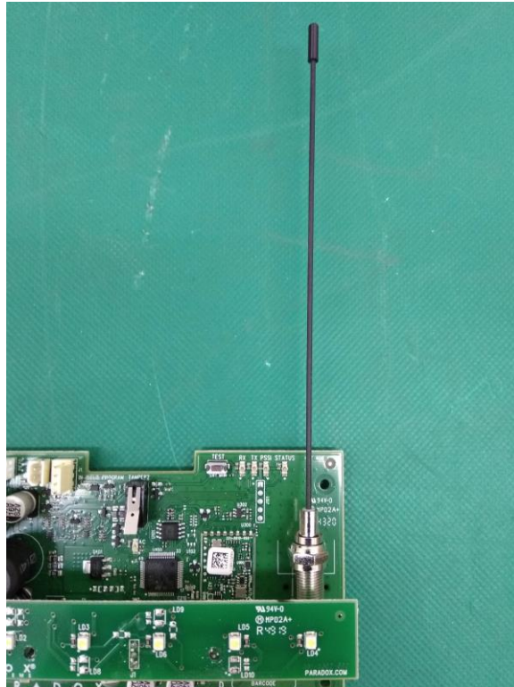
Photograph No.3 Antenna assembly
