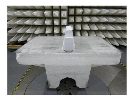
Photograph No.4 Setup for OBW measurements
