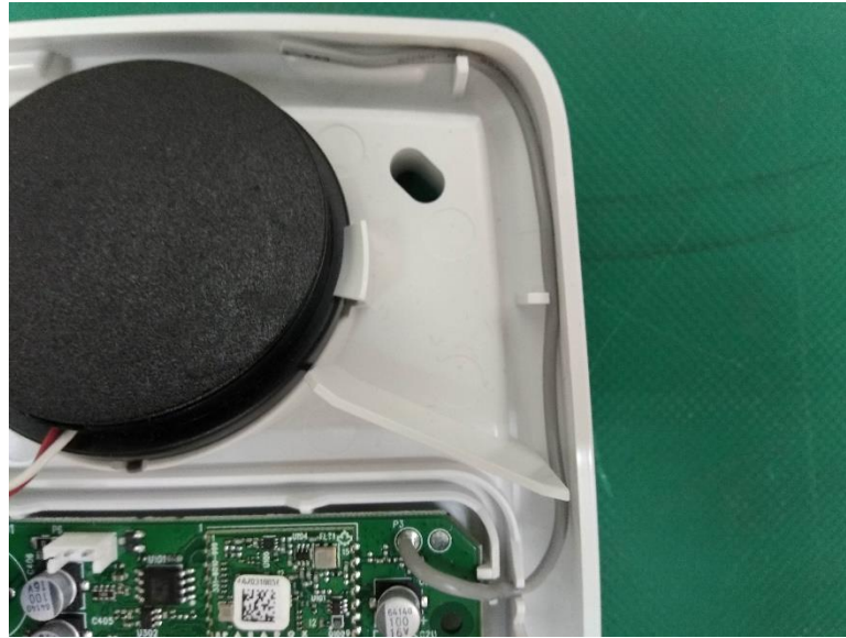
Photograph No.3 Antenna assembly
