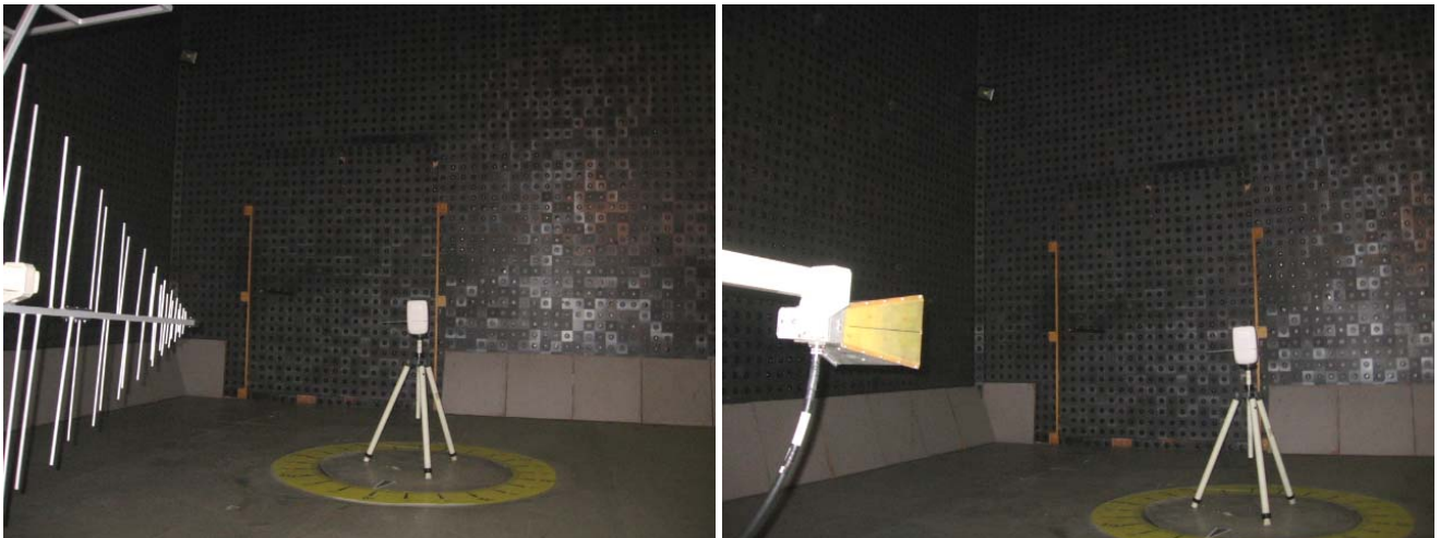
Photograph 8.1.1 Setup for radiated emission measurements
