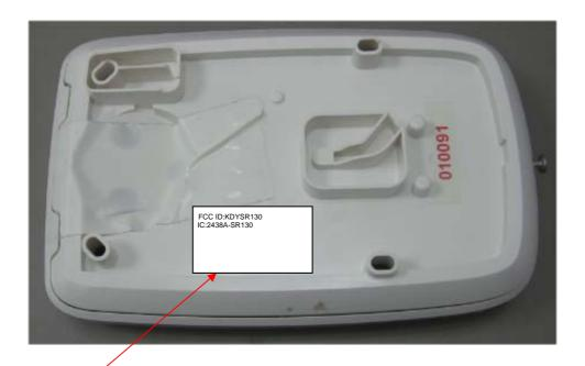
Label with FCC ID:KDYSR130 and IC:2438A-SR130 will be located at the rear side panel. The statement according to FCC part 15 §15.19(a)(3) is placed in User Manual, page 2 (Application exhibit User\_manual\_26426).
