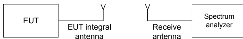
Figure 7.1.1 Setup for transmitter shut down test
