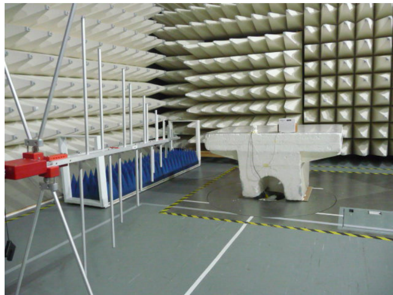
Photograph 7.2.1 Setup for radiated emission measurements
