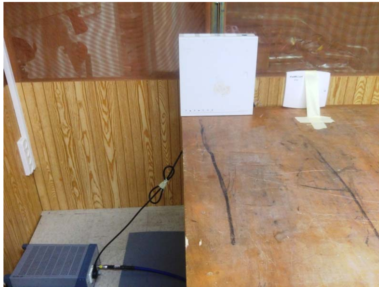
Photograph 7.1.1 Setup for conducted emission measurements
