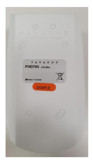
Label with **FCC ID:KDYPMD75N and IC:2438A-PMD75N** will be located here. The statement according to FCC part 15 §15.19(a)(3) is placed in User Manual, page 2 (Application exhibit User\_manual\_42332).
