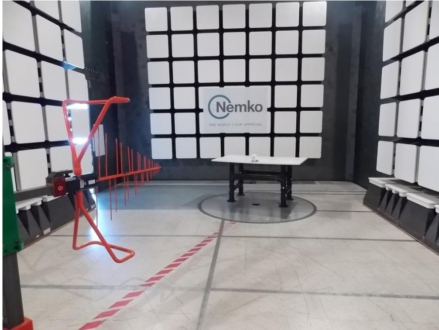
Figure 8.2-2: Emissions setup photo
