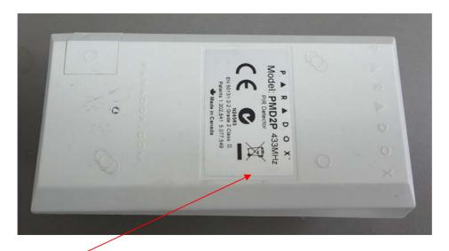
Label with FCC ID:KDYMGPMD2P and IC:2438A-MGPMD2P will be located at the rear side panel. The statement according to FCC part 15 §15.19(a)(3) is placed in User Manual, page 2 (Application exhibit User\_manual\_25766).
