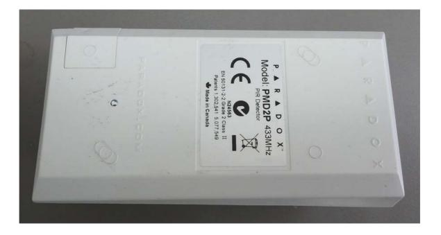
Photograph No.2 PMD2P PIR detector rear side view
