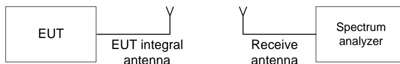
Figure 7.1.1 Setup for transmitter shut down test
