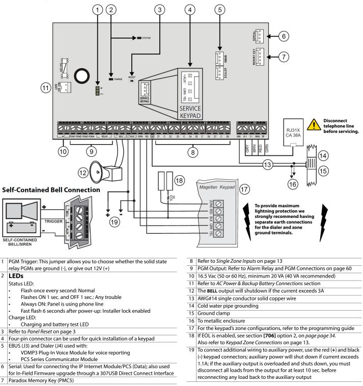
The sum of the current drawn from the BELL and AUX must be limited to 1.3A. Exceeding this limit will overload the panel power supply and lead to complete system shutdown.
