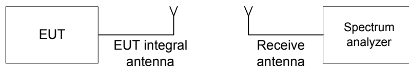
Figure 7.1.1 Setup for transmitter shut down test
