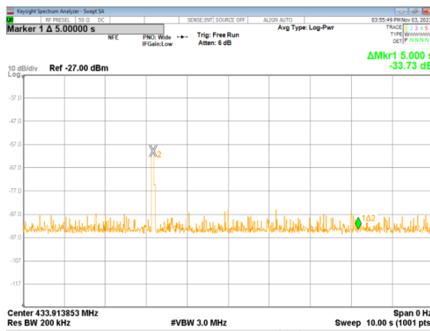
Plot 7.1.1 Transmitter shut down test result
