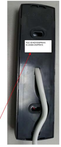
Label with **FCC ID:KDYDGPR915 and IC:2438A-DGPR915** will be located at the rear side panel. The statement according to FCC part 15 §15.19(a)(3) is placed in User Manual, page 2 (Application exhibit User\_manual\_25767).
