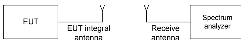
Figure 7.1.1 Setup for transmitter shut down test
