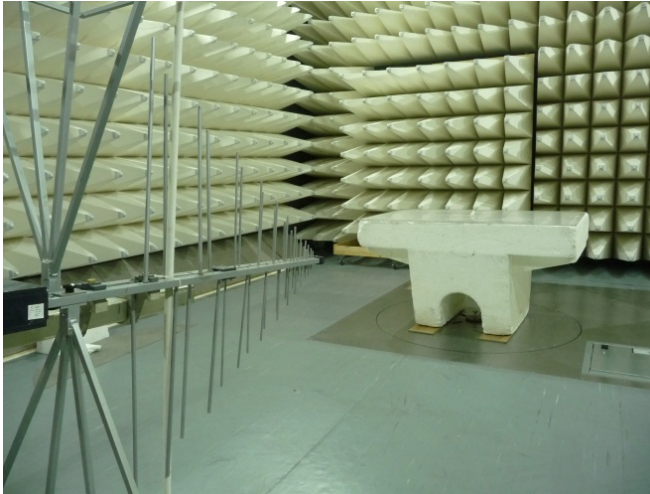
Photograph 8.1.2 Setup for radiated emission measurements, EUT close view
