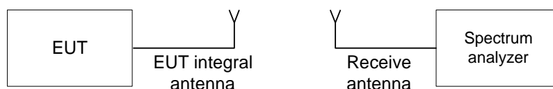
Figure 7.1.1 Setup for transmitter shut down test
